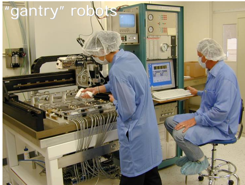
“gantry” robots automated module assembly and wire bonding
