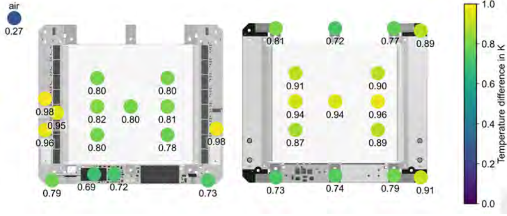
Figure 5.6: Heat map of the temperature differences on the 2S module's top side (left) and bottom side (right) the working point with a \text{CO}_2 temperature of -33.9^\circ\text{C} between only the 2S module powered and when the 2S module and all heating resistors are powered. The colored dots show the positions of the read out temperature sensors and the temperature differences in K are indicated.
